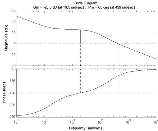
Figure 5 Bode characteristics for plant of Magnetic Levitation with designed controller
