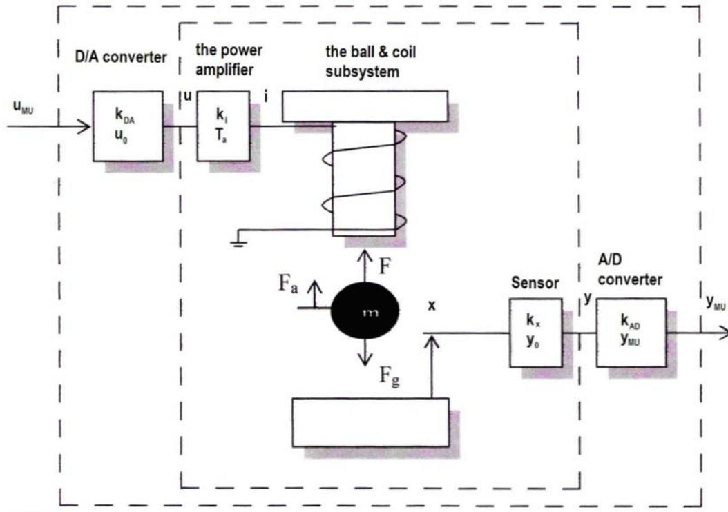
Figure 1: Scheme of the magnetic levitation model
