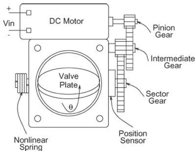
Figure 1.1: Electronic Throttle Body
