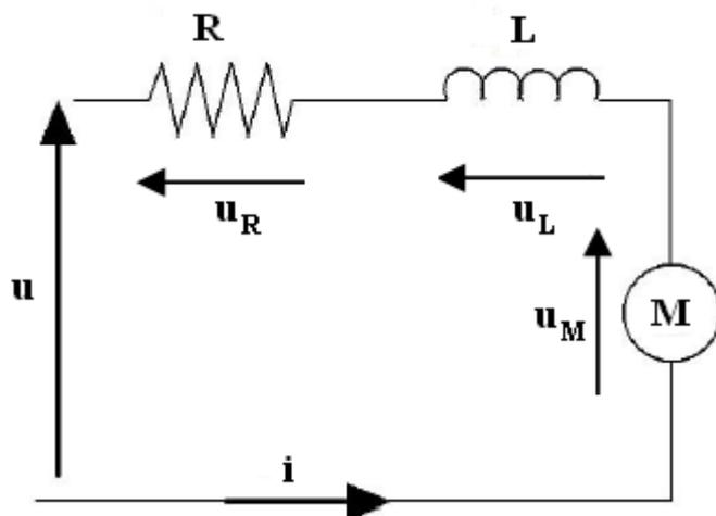
Figure 2.1: Electrical scheme of a DC motor
