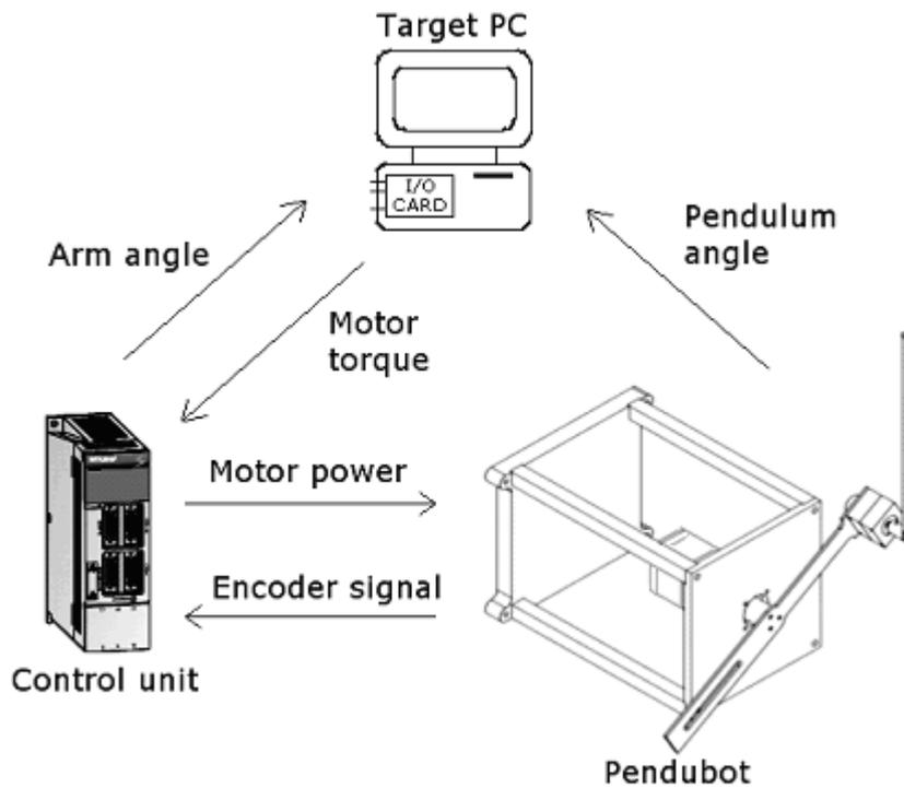
Figure 3: Pendubot hardware connection
