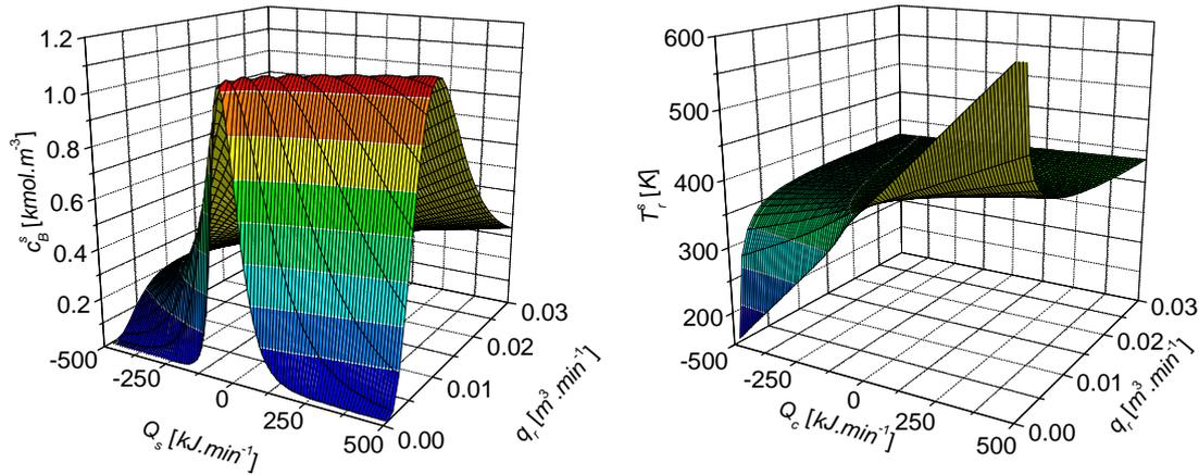
Figure 3: Steady-state values of the product's concentration,  $c_B^s$ , and the temperature of the reactant,  $T_r^s$ , for various heat removal,  $Q_c$ , and volumetric flow rate,  $q_r$
