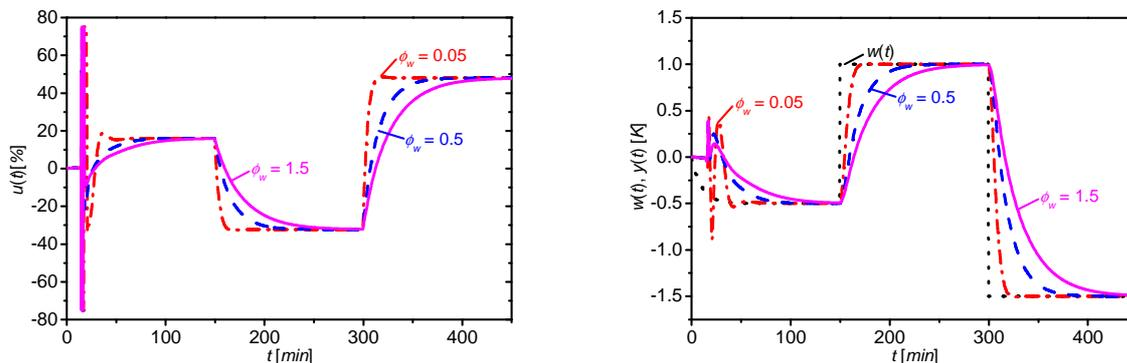
Figure 5: Course of input and output variables  $u(t)$  and  $y(t)$  for various weighting factors  $\phi_w$ , 1DOF configuration
