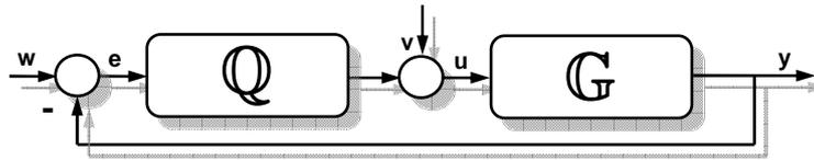
Figure 2: 1DOF control configuration
