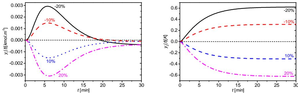
Figure 4: Dynamic analysis of outputs  $y_1 (c_B(t) - c_B^s)$  and  $y_2 (T_r(t) - T_r^s)$  for various step changes of the input heat removal,  $Q_c$
