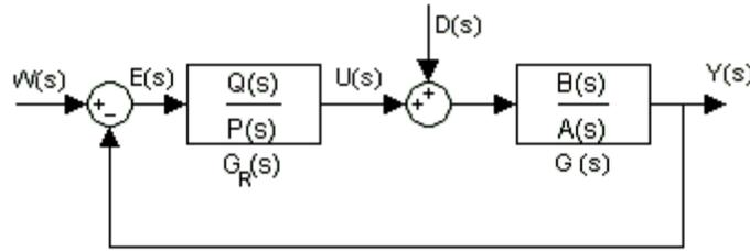
Figure 1: Simple feedback control loop
