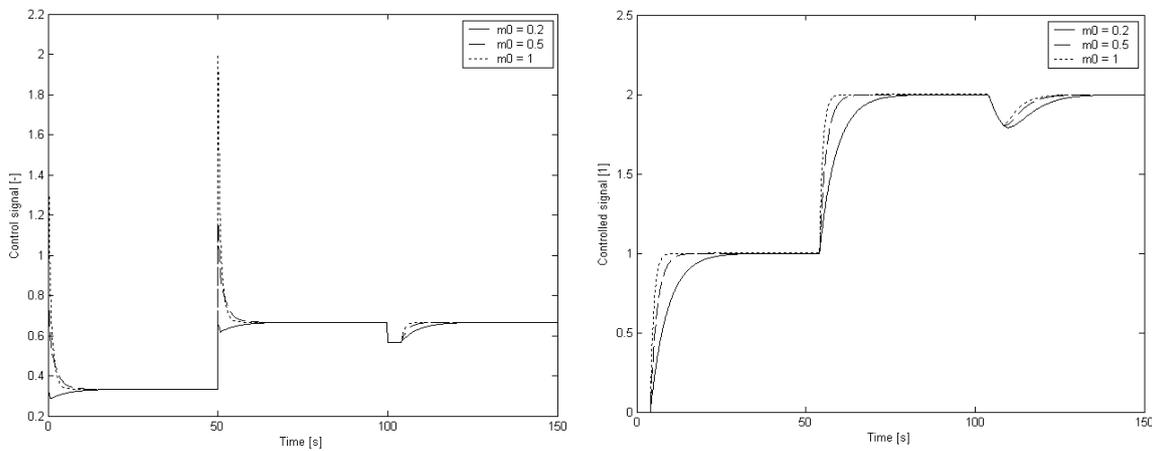
Figure 2: Closed-loop step responses for plant (27) and controller (28)
