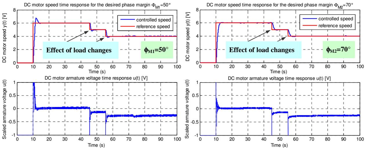
Fig. 5: DC motor closed-loop time responses for different phase margin values  $\phi_M$
