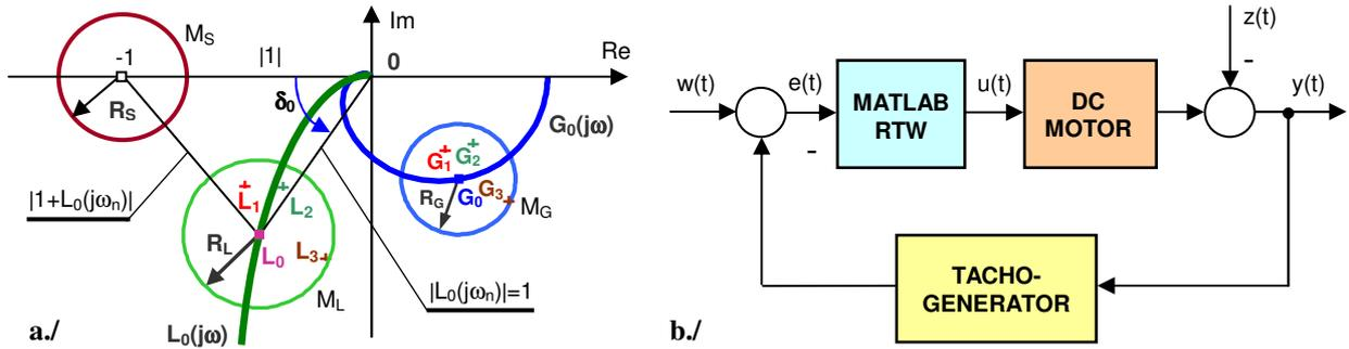
Fig. 4: a./ Dispersion circles  $M_G, M_L$  and the prohibited area delimited by the circle  $M_s$ , b./ Feedback loop of the DC motor
