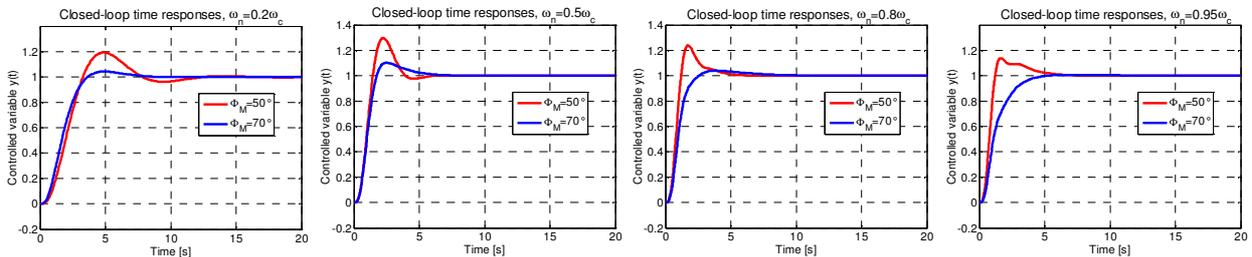
Fig. 3: Closed-loop step responses for both  $\phi_{M1}=50^\circ$  and  $\phi_{M2}=70^\circ$  on several identification levels  $\omega_{nk}$
