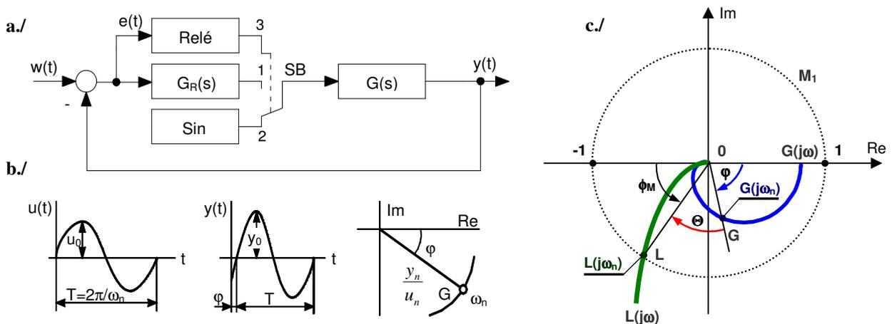
Fig. 1: a./ Feedback loop for the sine wave experimental method, b./ Identification procedure using the sine wave method, c./ graphical representation of the PID controller synthesis in the complex plane
