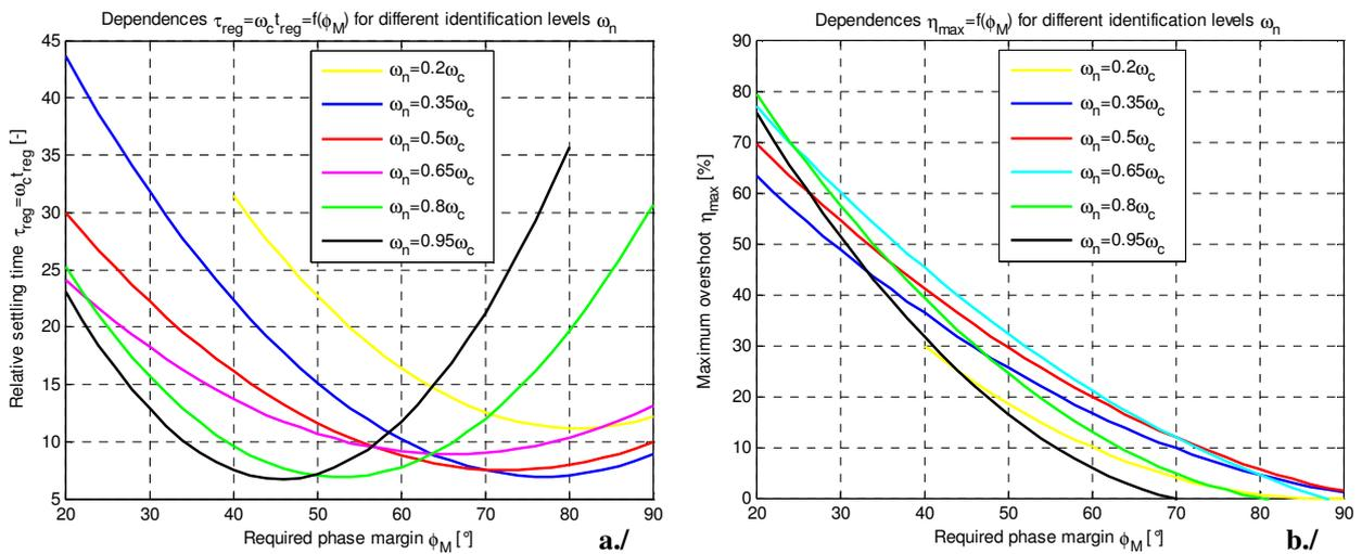
Fig. 2: Dependences: a./  $\tau_{reg} = \omega_c t_{reg} f(\phi_M)$ , b./  $\eta_{max} = f(\phi_M)$  for individual identification levels  $\omega_{nk}$ ,  $k=1,2,3,4,5,6$
