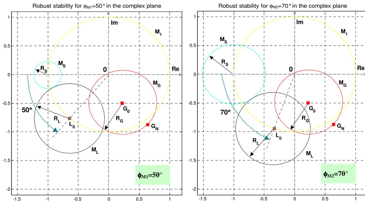
Fig. 6: Robust stability for different phase margins  $\phi_M$  depicted in the complex plane
