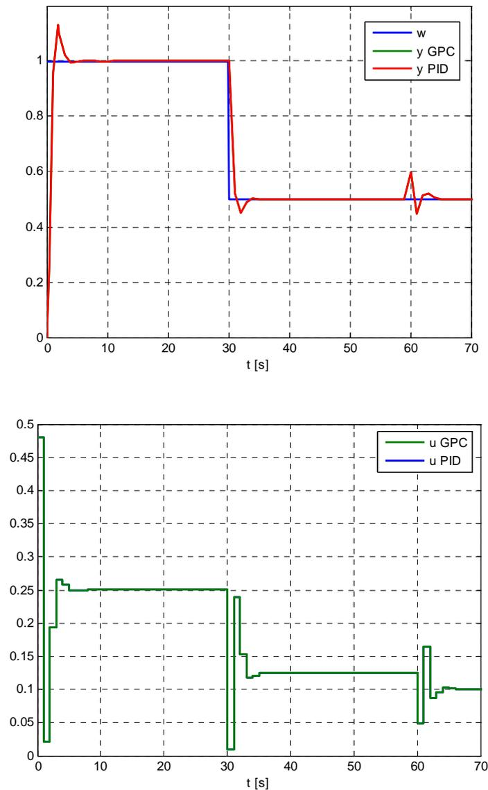
Figure 3 Comparison of GPC and PID control performances
