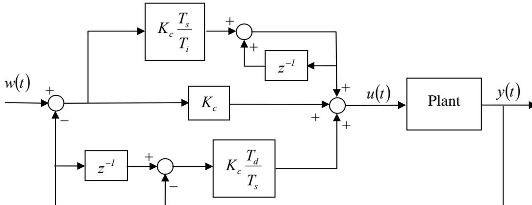
Figure 2 PID control structure
