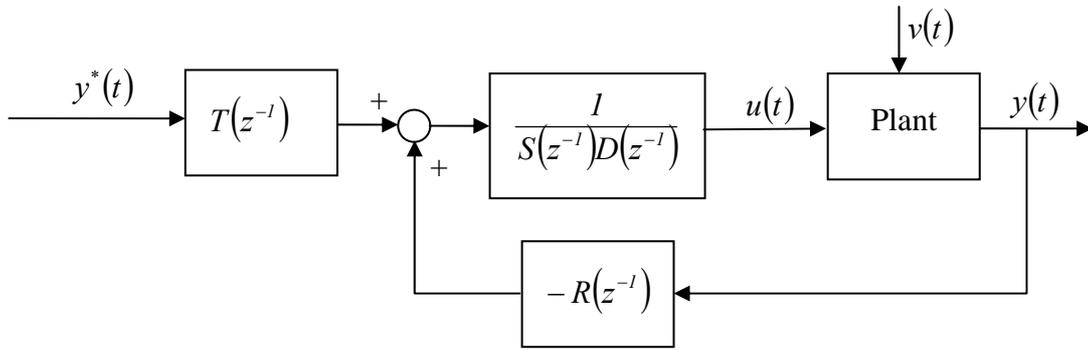
Figure 1 Standard pole-placement control structure
