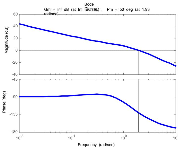
Figure 4: Bode characteristics for plant with desired controller
