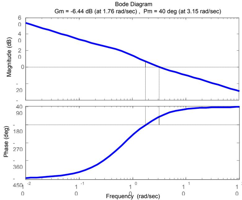
Figure 7: Bode characteristics for plant with desired controller
