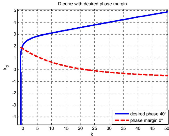
Figure 5: D-curve for parameters  $k$  and  $k_d$
