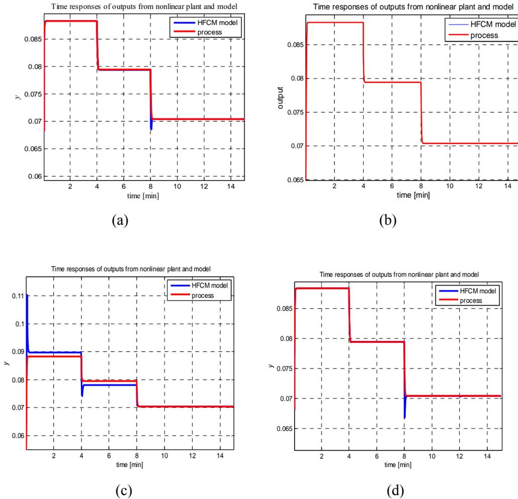
Figure 2: Time responses of output from the nonlinear plant and the HFNCM model with membership functions triangular (a), Gaussian (b), trapezoidal (c) and bell-type (d)
