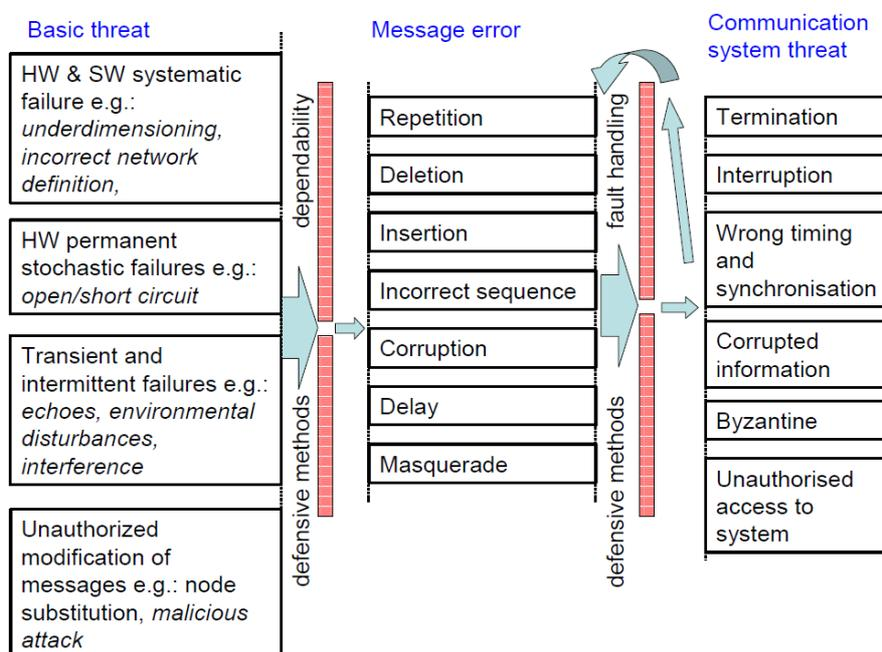
Figure 4: Fault model for wireless communications
