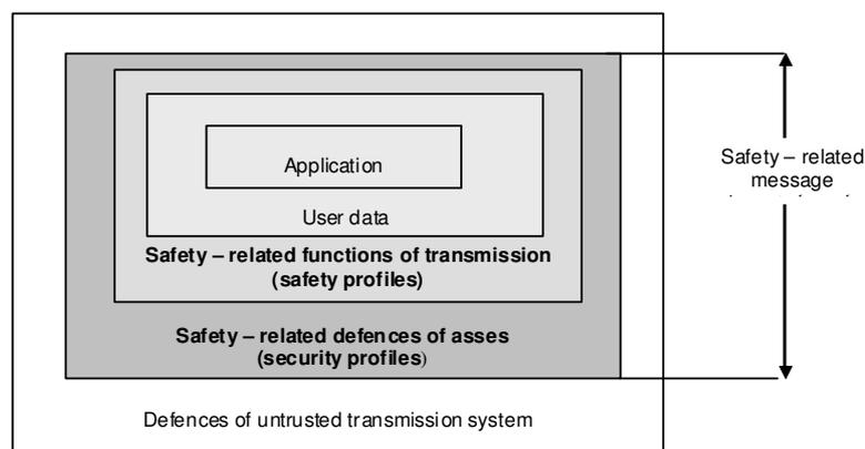
Figure 3: Model of safety - related communications in industrial applications
