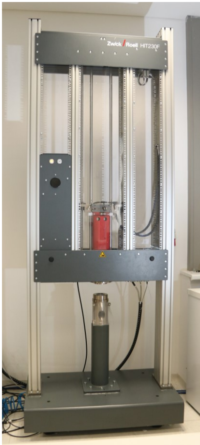
Fig. 1. Drop weight test machine used at Faculty of Applied informatics, TBU Zlin
