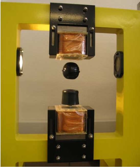
Fig. 3. The magnetic levitation system from INTECO, Ltd.
