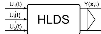
Fig. 2. Lumped input and distributed parameter output system with zero order hold units \{U_i(k)\}_{i=1,5}
