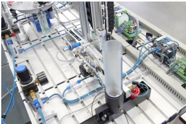
Fig. 1. The workpieces tray and the manipulator
