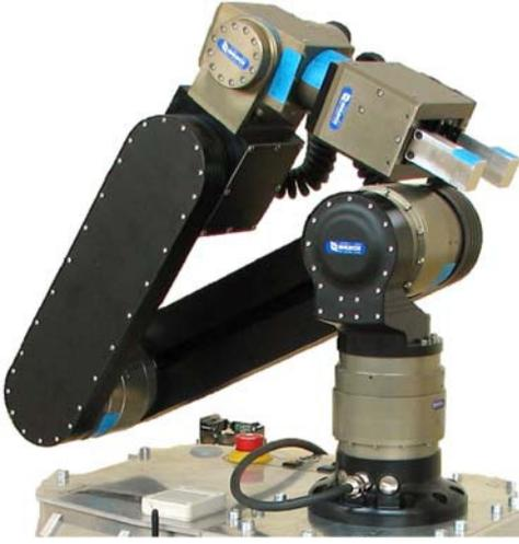
Fig. 3. 5 DOF articulated robot arm in detail [2].
