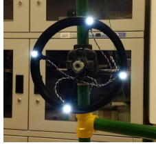
Fig. 2. Valve prototype and the attached LEDs.
