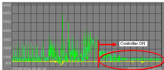
Fig. 9. Performance of the anti-slug control for one well.
