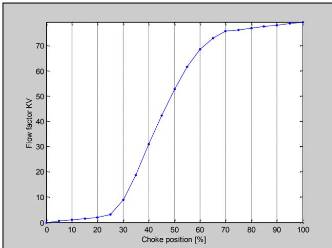
Fig 3: KV (CV) of the Drilling Choke
