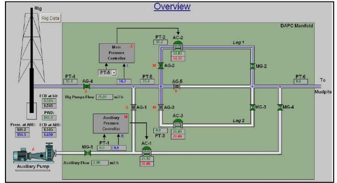
Fig 2. Prototype Control System Interface Overview Screen
