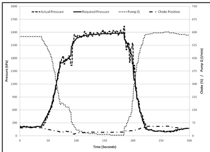
Fig 5: test #2 – Pump Stop / Start Sequence
