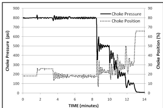
Fig 7: New Controller Test 4 – Gas Flow Stability Test
