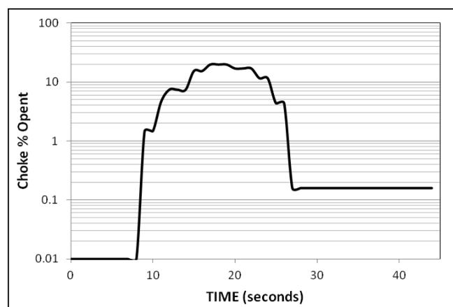
Fig 6b: Test #3 Choke position response to a gas kick
