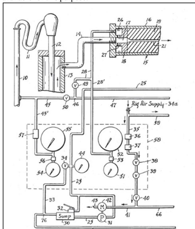
Fig 1: Automated choke control design - 1967
