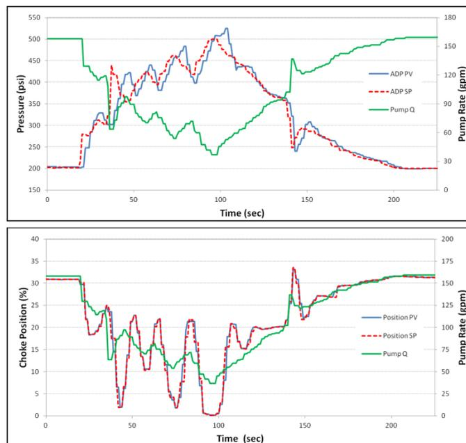
Fig 8a and 8b: Attempt to Destabilize Choke Controller
