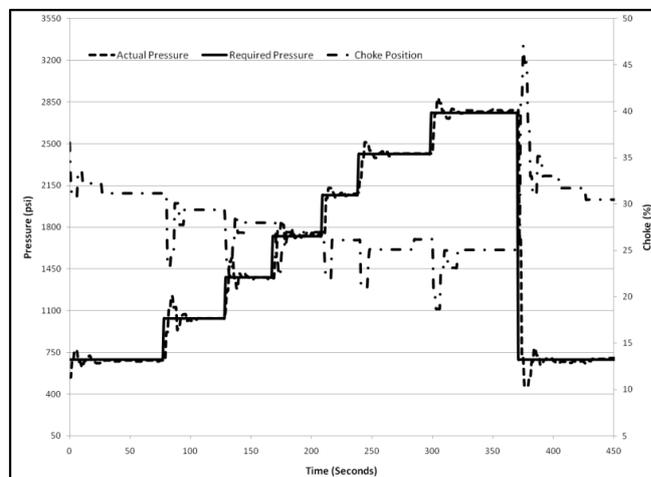
Fig 4: Test #1 – Manual Set Point Pressure Changes
