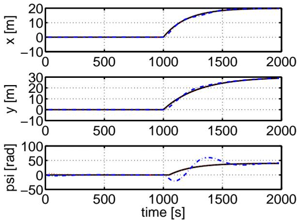
Fig. 5. Plot of the reference (black solid line) and estimated positions using the Multi-rate Kalman filter and the DTVSC (red dotted line) and the PID controller (blue dash-dotted line) in case of disturbances on the actuators
