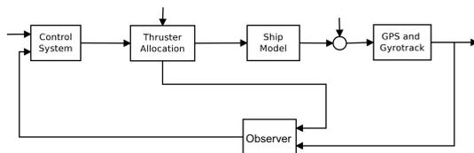
Fig. 1. Closed-loop DP system
