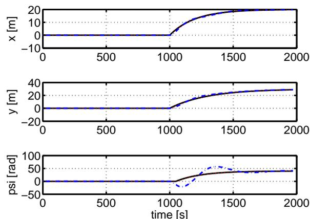
Fig. 4. Plot of the reference (black solid line) and estimated positions in the local geographical  $n$  frame using DTVSC controller (red dotted line) and the PID controller (blue dash-dotted line).
