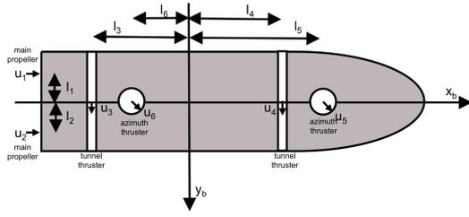
Fig. 2. Thrusters configuration for the offshore supply vessel
