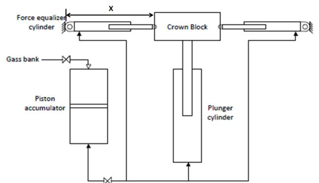
Fig. 3. The hydro-pneumatic system with a plunger cylinder and two force equaliser cylinders.
