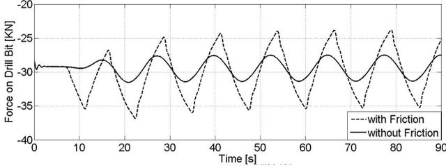
Fig. 6. Force on the Drill Bit where the passive compensation is used.
