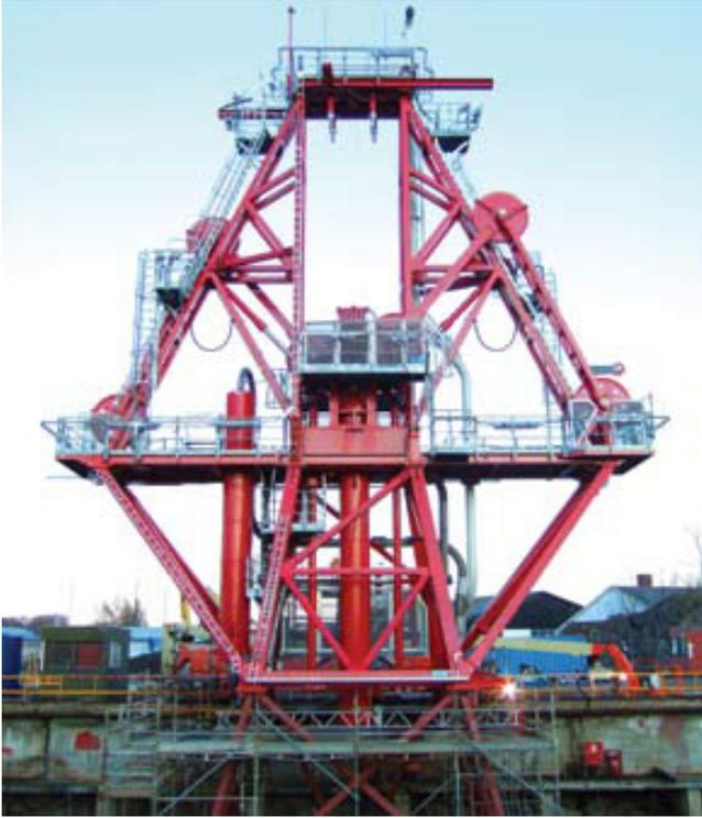
Fig. 1. The Drill String Compensator. The total height of the compensator equals 20 metres.
