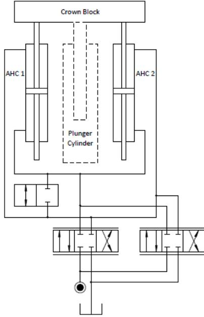
Fig. 4. The hydraulic system with active heave cylinders, two proportional valves and the bypass valve
