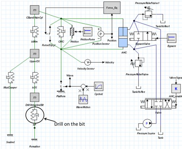
Fig. 5. 20-Sim based model of the drill string compensator without a control loop.
