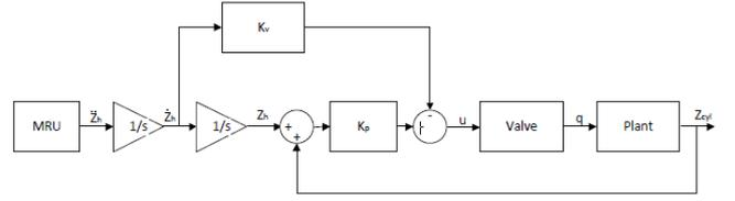
Fig. 7. Typical motion control.
