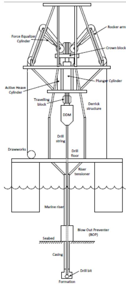
Fig. 2. Main arrangement of CMC drilling equipment.
