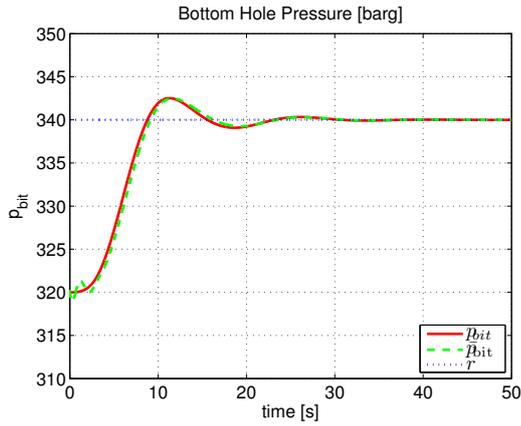
Fig. 5.  $p_{bit}$ ,  $\bar{p}_{bit}$ ,  $r$  for integrated estimator and controller
