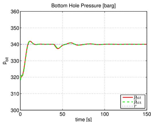
Fig. 11.  $p_{bit}$  during large parameter variation
