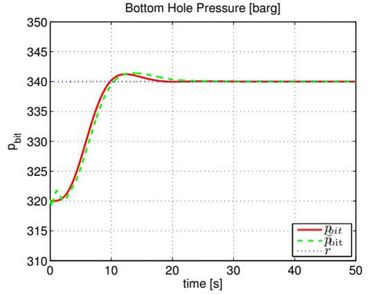
Fig. 2.  $p_{bit}$ ,  $\bar{p}_{bit}$ ,  $r$  for decoupled estimator and controller
