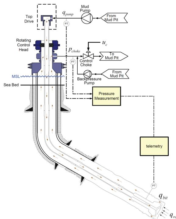
Fig. 1. MPD drilling process
