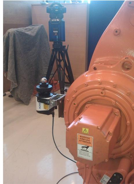
Fig. 3. FARO laser tracker used to calibrate the position of the laser scanner relative to the base of the robot.
