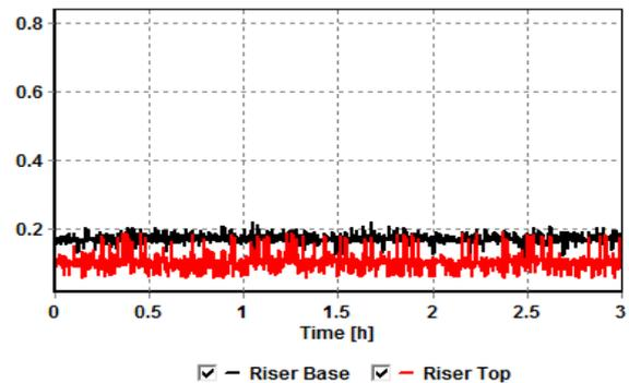
Fig.3. Holdup at the bottom and top of the riser with 1.282MMscf/d gas injection at the riser base
