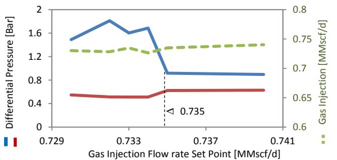
Fig.22. Bifurcation riser DP and gas injection flow rate against gas injection flow rate setpoint as CV
