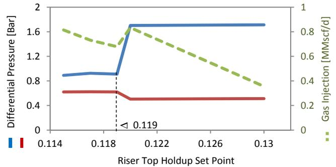
Fig.20. Bifurcation riser DP and gas injection flow rate against top holdup setpoint as CV
