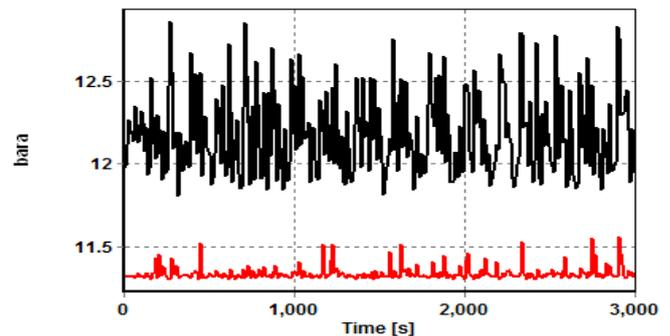
Fig.4. Riser bottom and top pressures without gas injection
