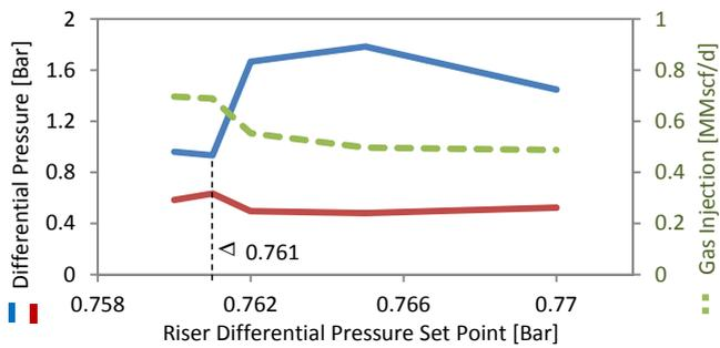
Fig.18. Bifurcation riser DP and gas injection flow rate against riser DP setpoint as CV
