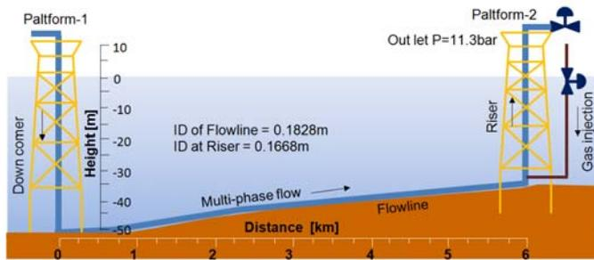
Fig. 1. Schematic diagram of pipeline with gas injection, pipeline profile as presented by Burke and Kashou (1996)
