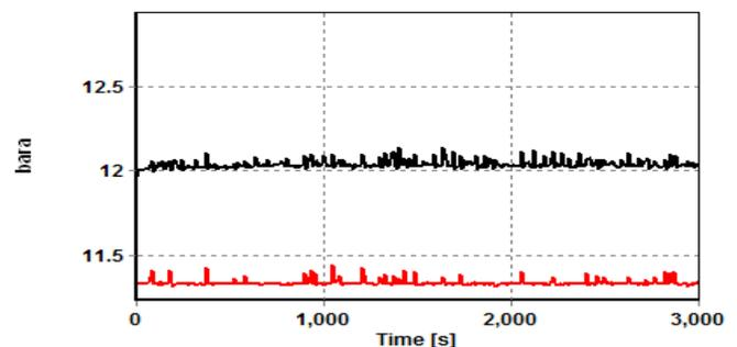
Fig.5. Riser bottom and top pressure at 1.282MMscf/d gas injection at the riser base.
