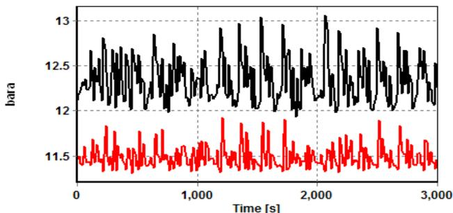
Fig.12 Pressure at the riser top and bottom at no gas injection
