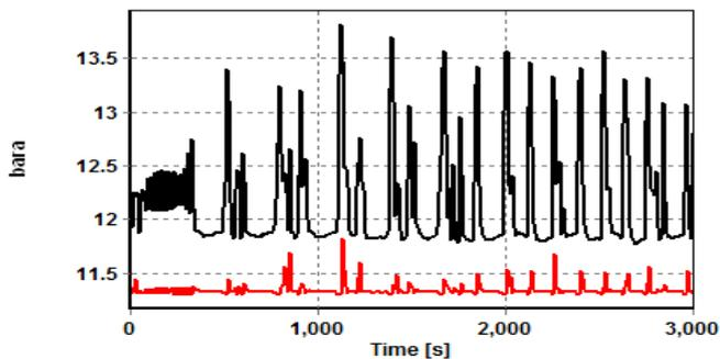
Fig.6. Riser bottom and top pressure at 1.282MMscf/d gas injection at the pipeline inlet
