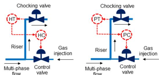
Fig.14. Holdup transmitter (HT) and pressure transmitter (PT) at the riser top.
