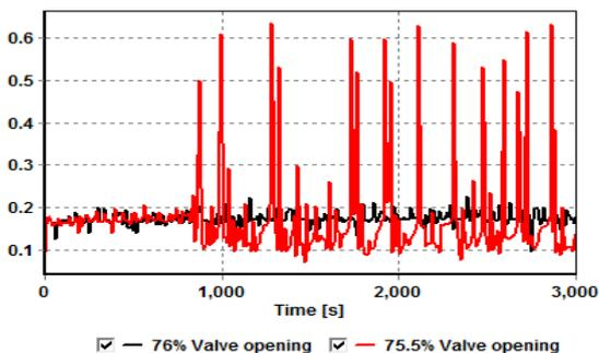
Fig.7. Holdup at the riser base at constant gas injection valve opening 76% and 75.5%
