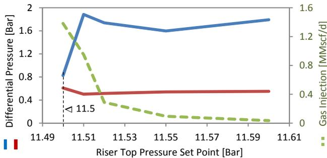
Fig.17. Bifurcation riser DP and gas injection flow rate against top pressure setpoint as CV
