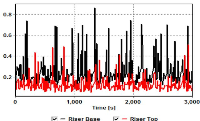
Fig. 2. Holdup at the bottom and top of the riser without gas injection
