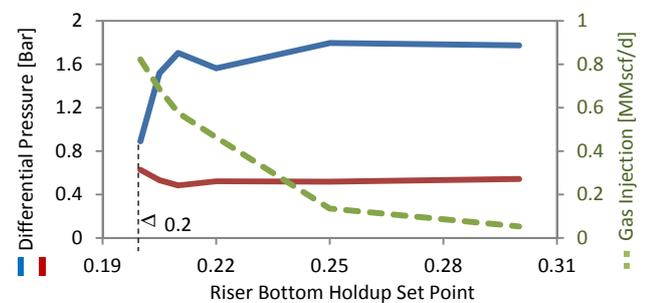
Fig.19. Bifurcation riser DP and gas injection flow rate against bottom holdup setpoint as CV
