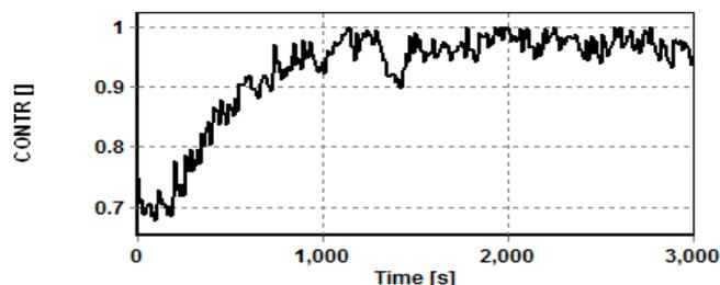
Fig.10. Controller response using pressure transmitter at the bottom of the riser, controller set point 12.03bara
