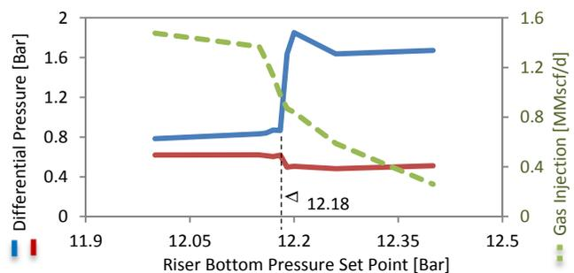
Fig.16. Bifurcation riser DP and gas injection flow rate against bottom pressure setpoint as controlled variable (CV)
