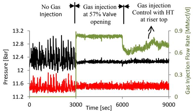
Fig.21. Pressure at the riser base and top and gas injection flow rate
