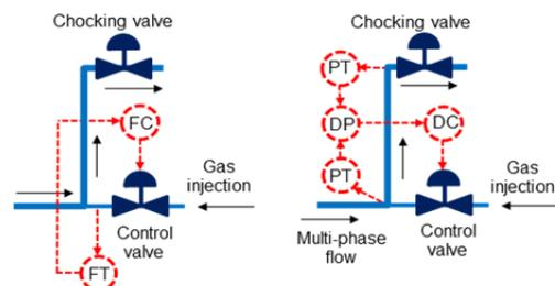
Fig.15. Flow transmitter (FT) downstream of the control valve and differential pressure (DP) across the riser.
