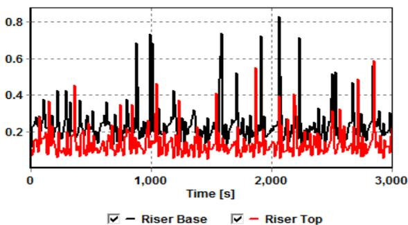
Fig.11. Holdup at the riser top and bottom at no gas injection
