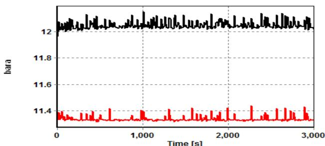
Fig.8. Riser bottom and top pressure at 76% gas injection valve opening
