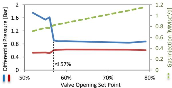
Fig.13. Bifurcation riser differential pressure (DP) and gas injection flow rate against constant valve opening
