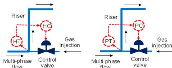
Fig.9. Holdup transmitter (HT) and pressure transmitter (PT) at the riser base.
