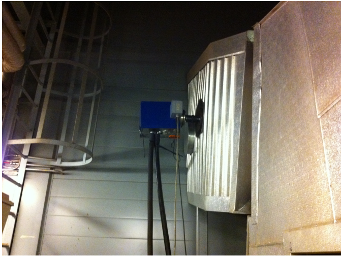
Fig. 5. Measurement set-up of the FT-IR analyzer in the flue gas duct
