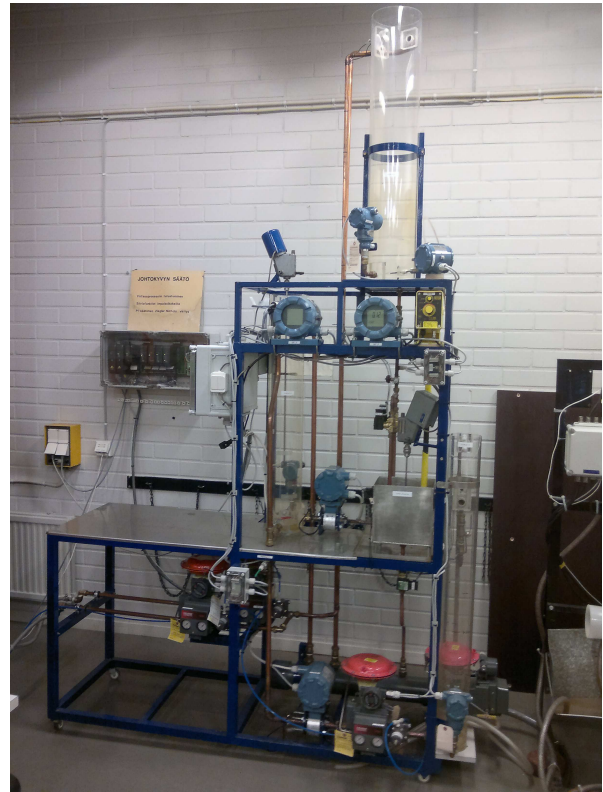
Fig. 1. The three tank system.
