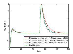
Fig. 8. Responses for PI-control of  $g = e^{-s}/s$  (E3).
