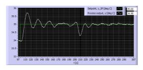
Figure 9: Ziegler-Nichols' Process Reaction Curve method: Responses in the control system.
