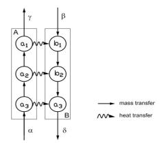
Figure 1: Model of the counter current double pipe heat exchanger with n equal three stages
