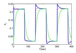
Fig. 15. Red dash line is the reference signal, the blue one is the QFT controller and the green one is the sliding mode controller response.  $x_1(0) = 0.05, x_2(0) = 0.3$
