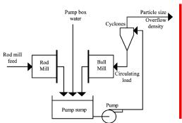
Figure 2. Grinding circuit, Lestage et al. 2002.
