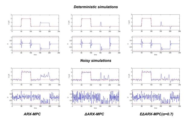
It is clearly seen on the figure that only the  $\Delta$ ARX and the E $\Delta$ ARX models can give offset free tracking. The output trajectories resulting from these two models are very similar but the E $\Delta$ ARX model give a less aggressive control action.
