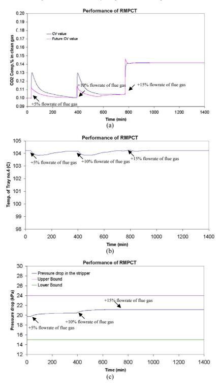
Fig. 7- a:  $CO_2$  content in clean gas stream, RMPCT has given up controlling of  $CO_2$  content in +15% of the disturbance, b: Temperature of tray no.4 in the stripper is always in its setpoint c: pressure drop of stripper
