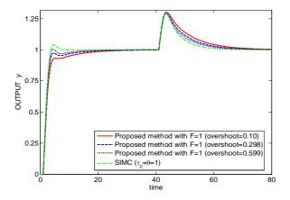
Fig. 6. Responses for PI-control of  $g = e^{-s}/(5s+1)$  (E1).
