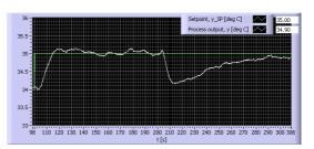
Figure 13: Tyreus-Luyben's method: sponses in the control system
