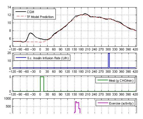
**Fig. 1.** Identification results for one subject. The TF model prediction is infinite-step. The experimental inputs included an unbolused meal at trial time 0 min, a bout of moderate exercise at trial time 150 min, and a correction bolus at trial time 300 min.
