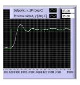
Figure 16: Sham's Setpoint method: The responses with a P-controller with gain  $K_{c0}=1.8$
