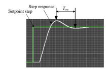
Figure 18: Reading off the time between the first overshoot and the first undershoot of the step response with P controller
