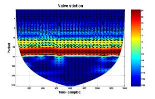
Fig. 9. Cross wavelet transform plot between u and  $y_p$  when the oscillation is only due to valve stiction.
