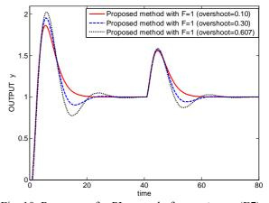
Fig. 10. Responses for PI-control of  $g = e^{-s}/(5s-1)$  (E7).
