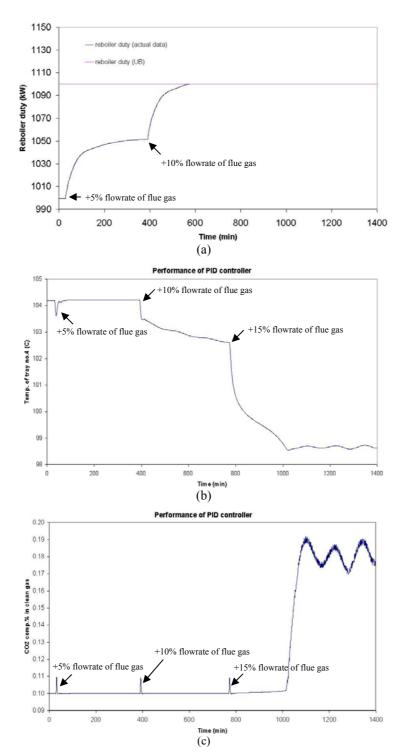
Fig. 3- a: saturation of reboiler duty when the flowrates of flue gas increases to +10%, b: when reboiler duty is saturated, by increasing feed flow to +15%, temperature of tray no.4 decreases significantly, c: instability of the process when flowrate of flue gas increases +15%
