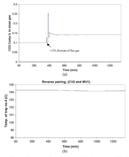
Fig. 6- By reverse pairing and giving up controlling the  $CO_2$  content in the clean gas when reboiler duty is saturated, control structure is stable when flue gas increases  $\pm 15\%$
