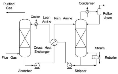
Fig.1- Absorption/Stripping CO<sub>2</sub> capturing process [2]
