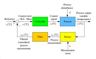
Figure 2: Block diagram of the temperature control system
