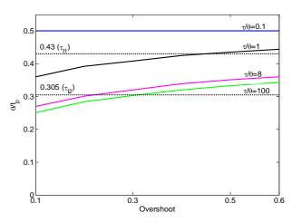
Fig. 5. Ratio between delay and setpoint overshoot peak time  $(\theta/t_p)$  for P-only control of first-order with delay processes (solid lines); Dotted lines: values used in final correlations.
