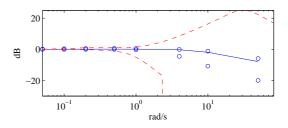
Fig. 12. The blue curve is nominal plant, the small circles show the uncertainty in the template, and the red envelope is the servo specification.
