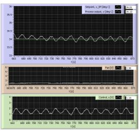
Figure 6: Skogestad's method: Responses with loop gain increase of 2.4
