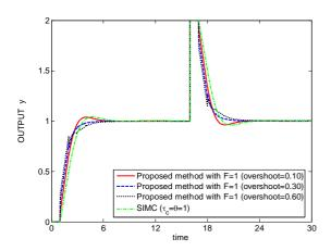
Fig. 7 Responses for PI-control of  $g = e^{-s}$  (E2).
