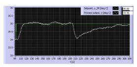
Figure 17: Sham's Setpoint method: The responses in the control system
