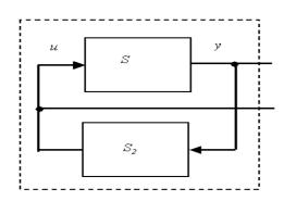
Fig. 4. General feedback control composition
