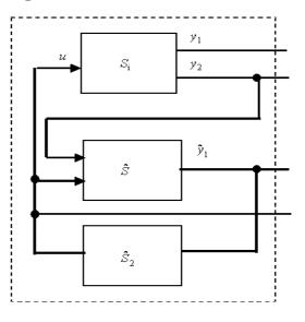
Fig. 6. State feedback with observer
