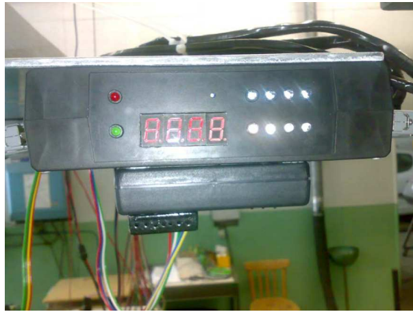
Fig. 5.15 Case with converters and security circuits
