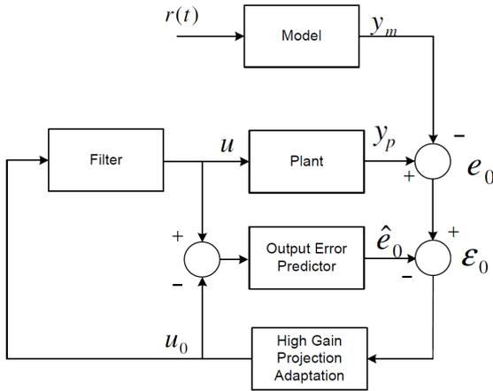
Fig. 4. Extended BMRAC (eBMRAC) block diagram
