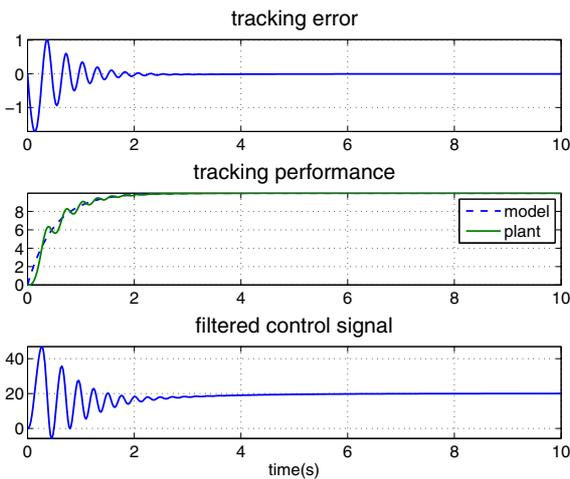
Fig. 12. eBMRAC step response for unknown  $K_p$  in Example 2
