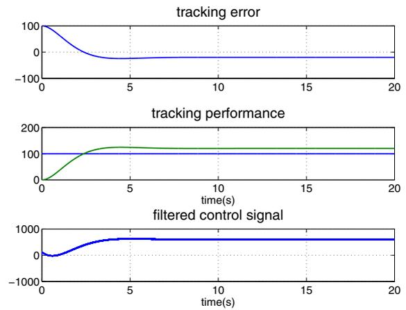
Fig. 9. L1-AC step response for unknown input gain in Example 2
