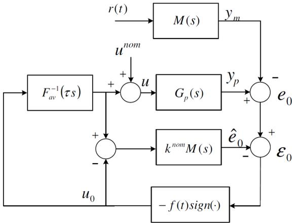
Fig. 2. Smooth sliding control block diagram
