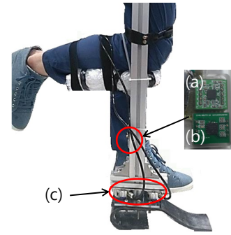
Fig. 3. Experimental device for detection of a gait pattern and an orientation angle of the device; (a) gyroscope, (b) accelerometer, and (c) load cells.
