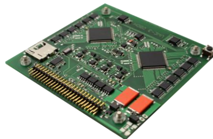
Fig.8. The Onboard Data Handling board with the two microcontrollers in hot redundancy
