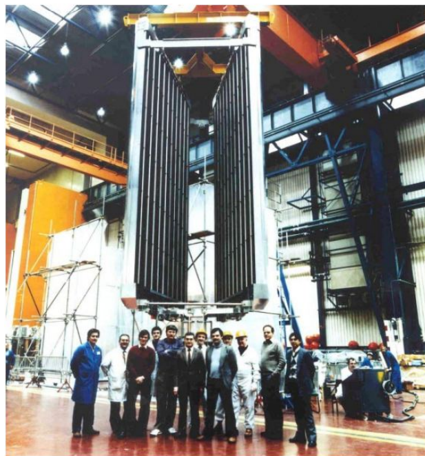
Fig. 1. The NBI cryopump panels prior to installation, courtesy CCFE
