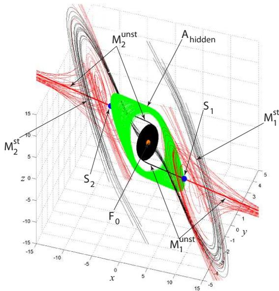
Fig. 5. Hidden chaotic attractor ( $A_{\text{hidden}}$  — green domain) in classical Chua circuit: locally stable zero equilibrium  $F_0$  attracts trajectories (black) from stable manifolds  $M_{1,2}^{\text{st}}$  of two saddle points  $S_{1,2}$ ; trajectories (red) from unstable manifolds  $M_{1,2}^{\text{unst}}$  tend to infinity;  $\alpha = 8.4562$ ,  $\beta = 12.0732$ ,  $\gamma = 0.0052$ ,  $m_0 = -0.1768$ ,  $m_1 = -1.1468$ .
