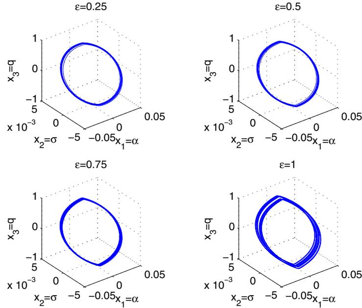
Fig. 8. Multistep localization of hidden oscillation:  $\varepsilon^j = j/4$ . At the last step (i.e.  $j = m$  in (5)) there is stable zero equilibrium point coexist with stable oscillation (hidden oscillation).
