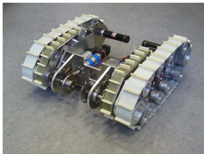
Fig. 3. Mechanical structure of Tracked MERLIN III.
