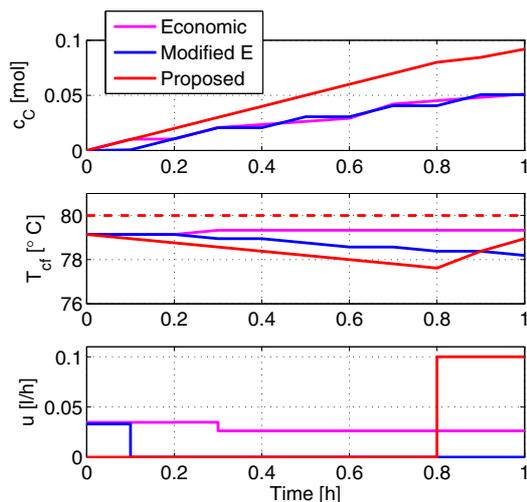
Fig. 3. Concentration  $c_C$ , temperature  $T_{cf}$  and control input  $u$  obtained from running robust optimal OED for different design criteria.
