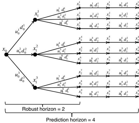
Fig. 1. Scenario tree representation of the uncertainty evolution for multi-stage NMPC.
