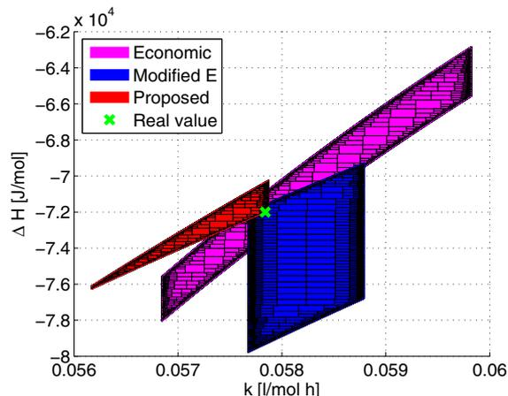
Fig. 4. Sets of guaranteed parameter estimates resulting from the measurements and control inputs obtained from optimal OED for different design criteria.
