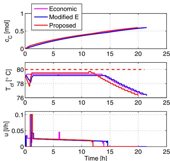
Fig. 5. Concentration  $c_C$ , temperature  $T_{cf}$  and control input  $u$  obtained from running multi-stage NMPC with a scenario tree generated with parameter bounds obtained by the guaranteed parameter estimation for different OED design criteria.
