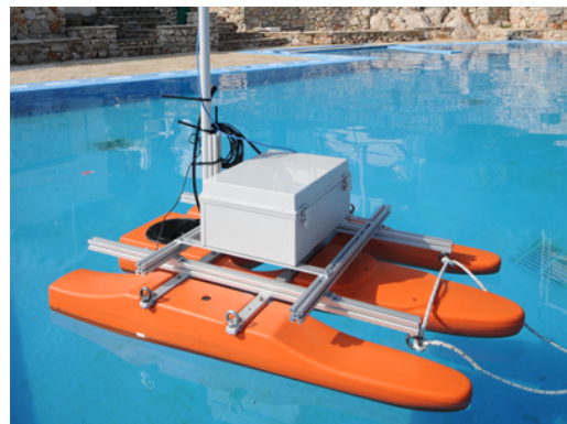
Fig. 2. Trimaran sampling platform during pool trials
