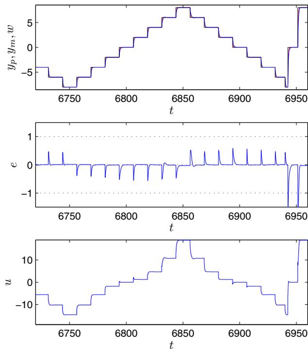
Fig. 3. The proposed evolving approach – time plots of  $y_p$ ,  $y_m$ ,  $w$  (upper figure), tracking error (middle figure), and the control signal (lower figure)
