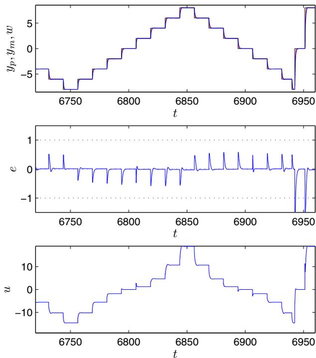
Fig. 1. The approach with fixed membership functions – time plots of  $y_p$ ,  $y_m$ ,  $w$  (upper figure), tracking error (middle figure), and the control signal (lower figure)
