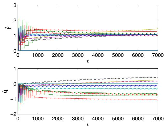
Fig. 2. The approach with fixed membership functions – time plots of feedforward and feedback control gains
