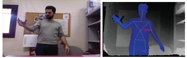
Fig. 4. Visual Demonstrations Teaching of a Skill: (left) A human teacher performs a demonstration. (right) The generated skeleton of the human recorded demonstration.
