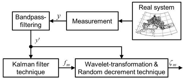
Fig. 12 Scheme of the coupling of KFT and WTRD
