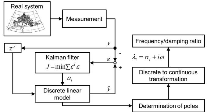
Fig. 3. Principle scheme of the Kalman filtering technique
