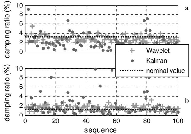
Fig. 8 Damping ratio estimation of  $\zeta_1$  (a) and  $\zeta_2$  (b) with the KFT and the WT
