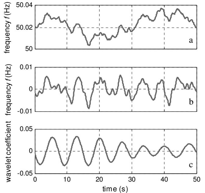
Fig. 5 Frequency signal (a), corresponding bandpass filtered signal (b) and wavelet transformed signal (c) for the oscillation mode with the frequency  $f=0.134\text{ Hz}$
