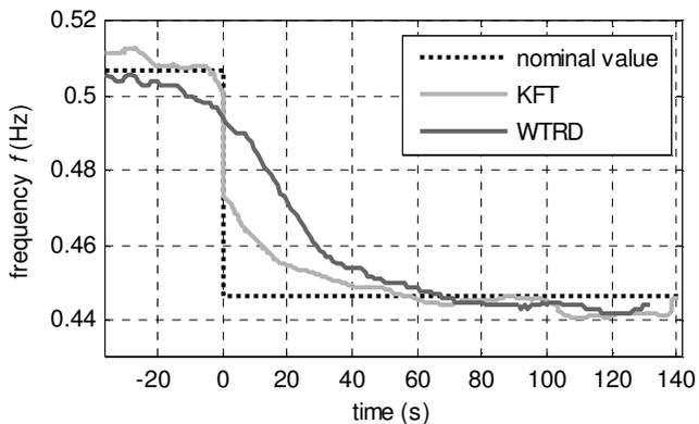
Fig. 11 Comparison of WTRD and KFT detecting a change in frequency
