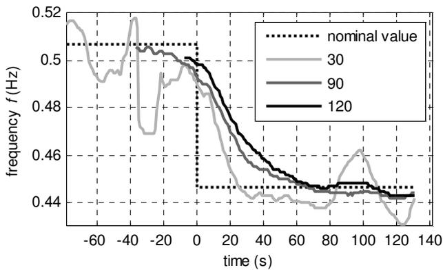
Fig. 10 Detection of a change in frequency due to line tripping with the WTRD technique using window lengths of 30, 90, and 120 seconds
