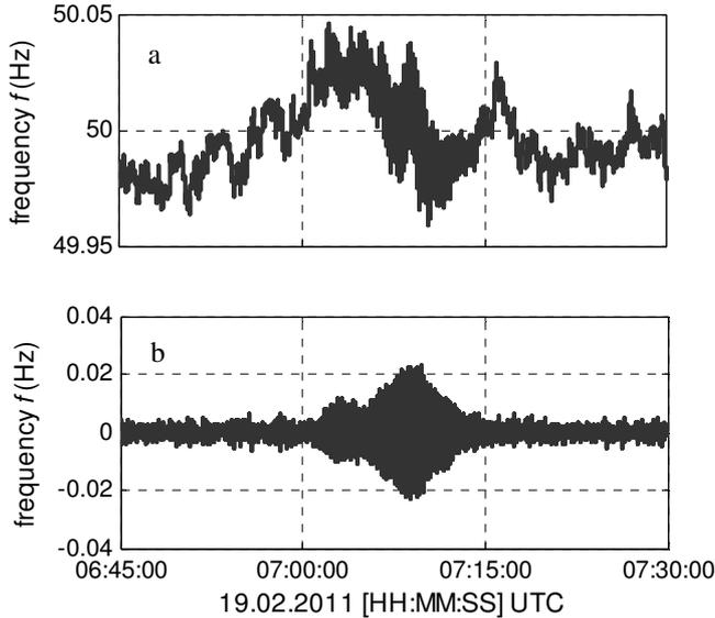
Fig. 14 Undamped oscillations in the frequency measurements of Aalborg, Denmark (a) and the filtered signal (b)
