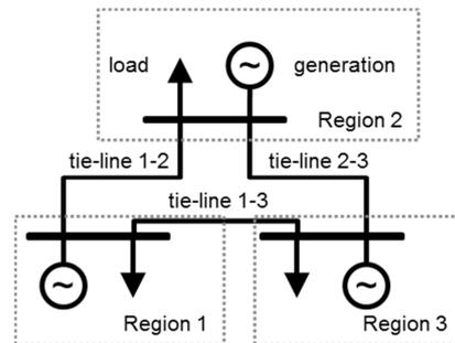
Fig. 9 Structure of the synthetic power system
