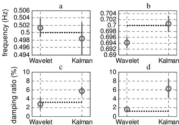
Fig. 7 Average and standard deviation of  $f_1$  (a),  $f_2$  (b),  $\zeta_1$  (c), and  $\zeta_2$  (d), each with the KFT and WTRD plus the nominal value (dotted line)
