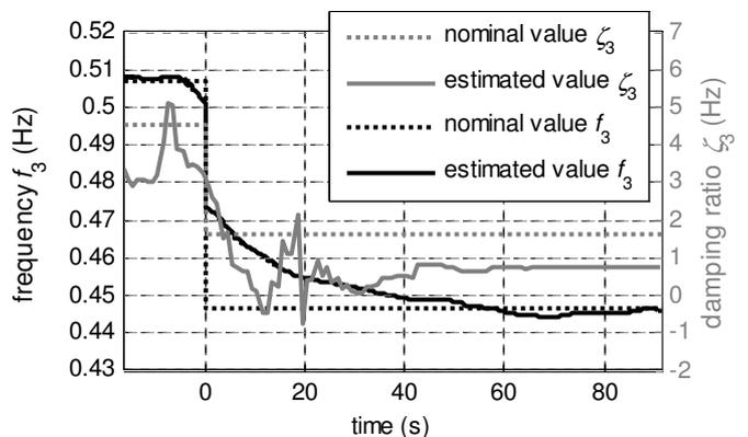
Fig. 13 Detection of change of dynamic parameters due to line tripping with use of a coupled method of KFT and WTRD
