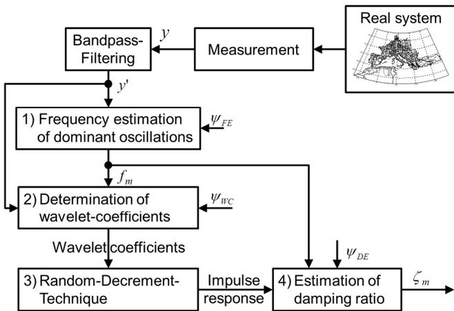
Fig. 4. General principle of the wavelet transformation technique
