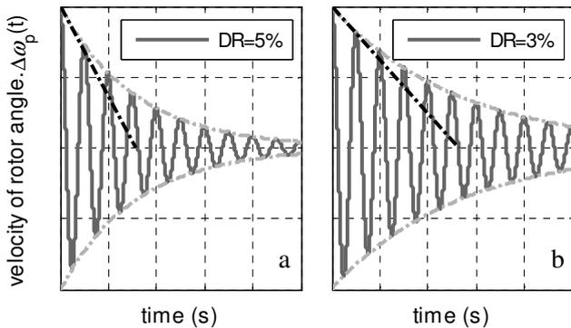
Fig. 2 Two decaying oscillations with damping ratio of 5% (a) and 3% (b).
