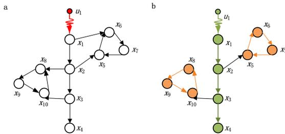
Fig. 2. Structural controllability of a network. **a**, A sample network of ten state nodes and one control node. **b**, The network is spanned by cacti which can be decomposed into node-disjoint stems (in green) and cycles (in yellow), indicating it is structurally controllable. For the definitions of cacti, stem and cycle, please refer to (Lin (1974)).
