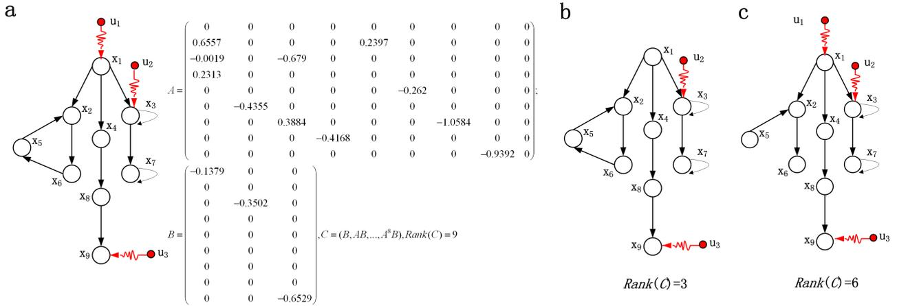
Fig. 1. An illustrative example on how a network loses its controllability due to malicious attacks or random failures. **a**, A directed weighted network with nine state nodes and three control nodes whose controllability matrix has the full rank. **b**, When control node  $u_1$  breaks down, the rank of  $C$  becomes 3, indicating the damaged network loses its controllability. **c**, When the link  $(x_6, x_5)$  breaks, it leads the rank of  $C$  to 6, losing its controllability.
