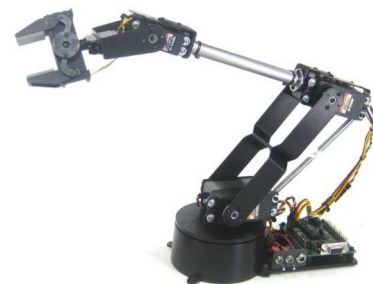
Fig. 5. Robotic arm and SSC-32 controller.
