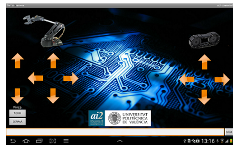
Fig. 12. Android application interface developed to control the platform.
