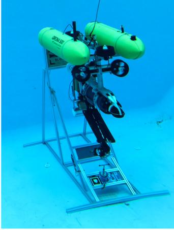
Fig. 1. Girona 500 I-AUV with a manipulator attached docked into the mock-up intervention panel.
