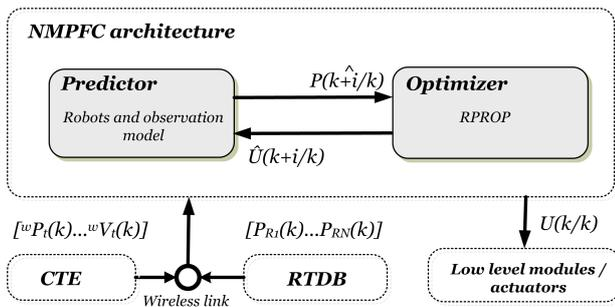
Fig. 2. Controller diagram for each robot.
