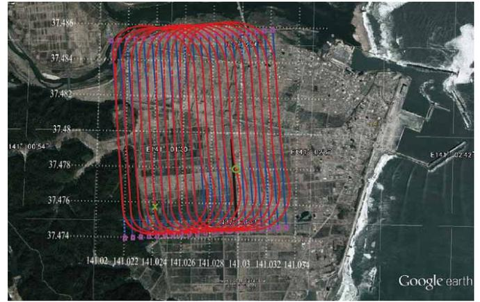
Fig. 6. Horizontal view of path-following for radiation monitoring demonstration (“x” and “o” respectively denote the autopilot engage and disengage points.)
