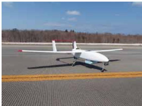
Fig. 1. UARMS (The blue box under the fuselage is a part of radiation measurement apparatus.)
