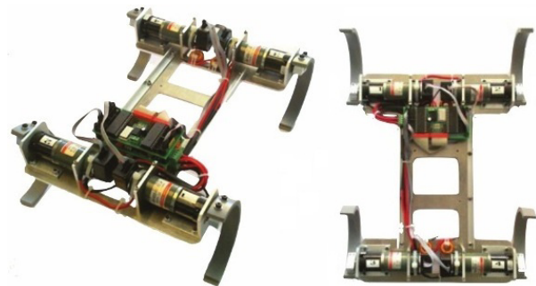
Fig. 1. Four-legged robot RQuad developed at Delft Center for System and Control, TU Delft.
