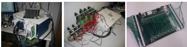
Fig. 1. First (Left), Second (Middle), and Third (Right) Analog Power System Emulator Prototypes Referred to in this Paper
