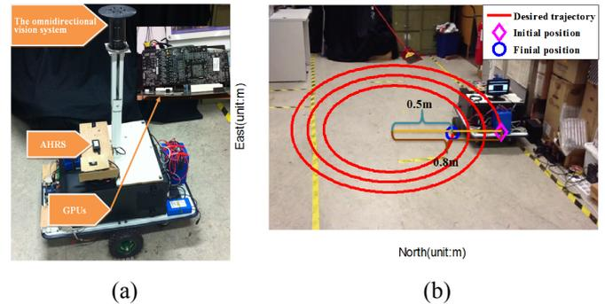
Fig. 2. The experiment setup: (a) The mobile robot. (b) The desired trajectory in an indoor environment.
