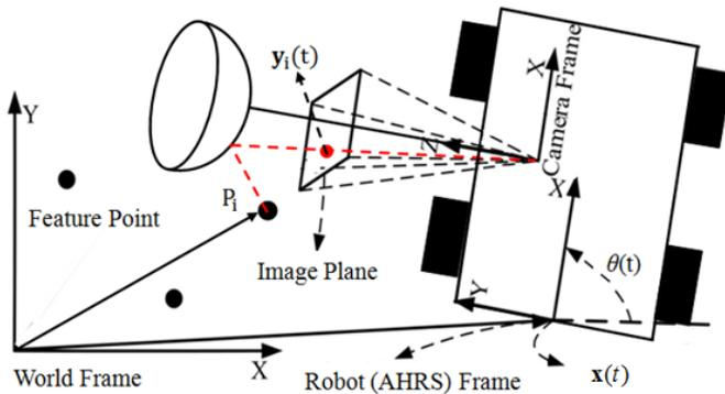
Fig. 1. The coordinate frames of the mobile robot.
