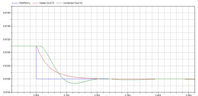
Fig. 9. Response to a humidity set point step with the conventional AHU of Figure 6 (red) and the DW-endowed one of Figure 7 (green).
