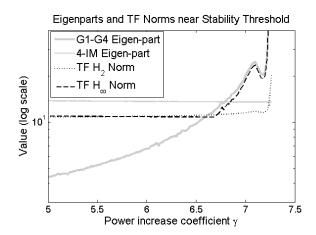
Fig. 2.  $H_2$  and  $H_{\infty}$  norms of the transfer function and two largest eigen-parts as functions of power increase coefficient  $\gamma$
