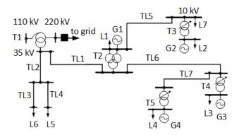
Fig. 1. One-line diagram power network: T1-T5, L1-L7, TL1-TL7, G1-G4 are equivalent transformers, loads, transmission lines and generators respectively
