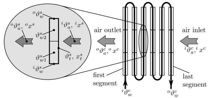
Fig. 3. Structure of the heating/cooling coil.
