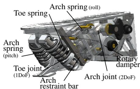
Fig. 5. Mechanical foot model
